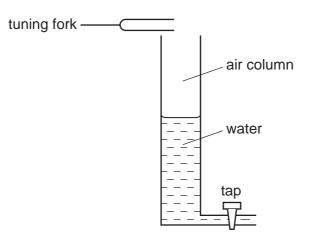
The tube is filled and then water is allowed to run out of it. The first two stationary waves occur when the air column lengths are  $0.14 \,\text{m}$  and  $0.42 \,\text{m}$ .
