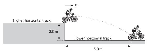
The cyclist travels a horizontal distance of 6.0 m in the air. Air resistance is negligible.
